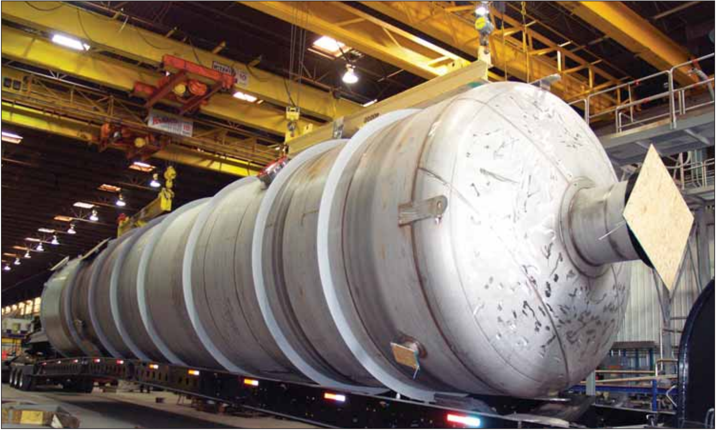
A 70-foot long vessel made of half-inch thick stainless steel being readied for shipment.
