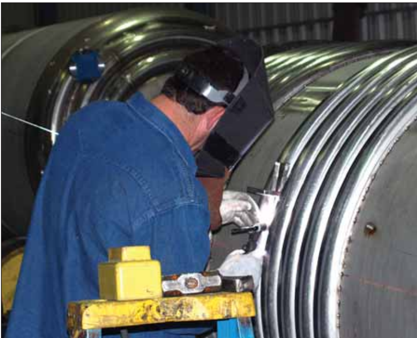
Welding dimpled jacket to a chemical vessel. Below: Welding half-pipe coil.
