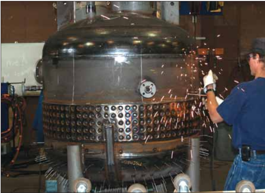
Welding dimpled jacket to a chemical vessel. Below: Welding half-pipe coil.
